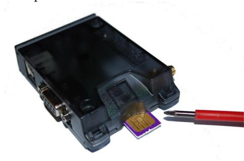
Insert the SIM card in the SIM card holder and push it back into the housing.
