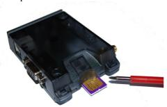
Insert the SIM card in the SIM card holder and push it back into the housing.
